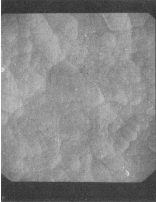
FIGURE 4 Scanning electron micrograph of the "Goretex" polymer after coating with 1.5 \mu\text{m} thick film of poly( p -xylylene) (5000 \times ).
